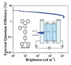
An intercrossed-excited-state (local exciton (LE) and charge transfer (CT)) character, which is identified based on the solvatochromic effect and density functional theory (DFT) calculations, endows the twisting donor-acceptor triphenylamine-imidazol molecule, TPA-PPI, with highly efficient, deep-blue electroluminescence. As one of the best results reported, the intercrossed excited state is thought to be beneficial for obtaining high-efficiency EL.
