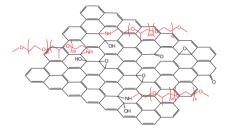
Covalently modified graphene is fabricated by grafting the end amine groups of a long-chain molecule with the epoxide groups of graphene platelets. These high C:O ratio platelets are produced by the ultrasonication and thermal treatment of a commercial graphite intercalation compound. Their epoxy nanocomposites show a low percolation threshold at 0.25 vol%.
