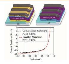
A comprehensive characterization and optical modeling of polymer solar cells is performed on a series of conventional and inverted structure devices to understand the effect of device geometry on photovoltaic performance. Excellent device performance could be achieved by optimizing the optical field distribution and spatial profiles of excitons generation within the active layer in these device configurations.
