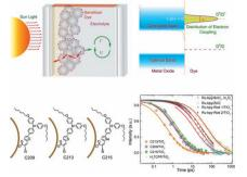
Initial nanointerfacial electron transfer dynamics are studied in dye-sensitized solar cells. The decay profiles, reflecting the electron transfer behavior, show a universal shape. In order to quantitatively comprehend the universal behavior, a static inhomogeneous electronic coupling model with a Gaussian distribution of local injection energetics is proposed in which only the electron injection rate is a variant.
