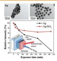
Localized surface plasmon (LSP) effects due to Ag and Ag@SiO<sub>2</sub> nanoparticles (NPs) are studied. GaN/InGaN lightemitting diode (LED) structures coated with the NPs exhibit enhanced photoluminescence efficiency as a result of coupling between the LSP and the LED active region. Compared with Ag NPs, Ag@SiO<sub>2</sub> NPs display a much higher optical stability with respect to long-term storage and annealing because of the protection of Ag by the SiO<sub>2</sub> shell.
