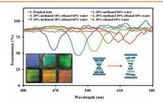
Alcohol-responsive, hydrogen-bonded, cholesteric liquid-crystal (CLC) networks are used for the detection of and distinction between ethanol and methanol molecules using a hydrogen-bridged CLC network with a controlled porosity. The reflecting color of CLC films has an obviously different response that is determined by the alcohol solution uptake.
