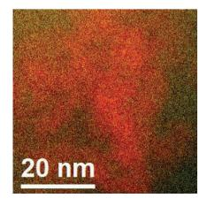
Ceria-zirconia solid solutions homogeneously undergo phase transformations from cubic to tetragonal structures. This is due to the initial intimate mixing of the constituent cations, as the energy-filtered transmission electron microscopy (EFTEM) image shows.
