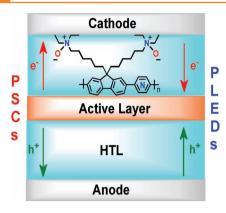
Alcohol-soluble neutral conjugated polymers with amino N-oxide functionalized side chains and different linkages of pyridinyl moieties in the main chain are synthesized as a cathode interlayer for polymer light-emitting diodes (PLEDs) and polymer solar cells (PSCs). High performance of PLEDs and PSCs is achieved by using these polymers as cathode interlayers, which indicates a promising pathway to PLEDs and PSCs with high efficiencies.
