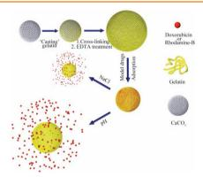
A "cast" strategy is applied to fabricate biodegradable and biocompatible gelatin microgels with a uniform size and porous structure. The manufacturing process involves no organic solvents and surfactants. Model drugs with a low molecular weight and positive charge can be loaded into the microgels via electrostatic interaction and release is automatically triggered by changing the salt concentration and pH, respectively.
